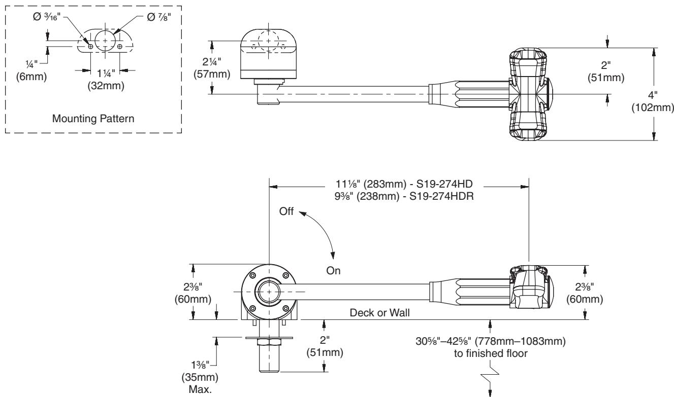
**Dimensions — S19-270JD, S19-270JW** (deck-mounted unit shown)
