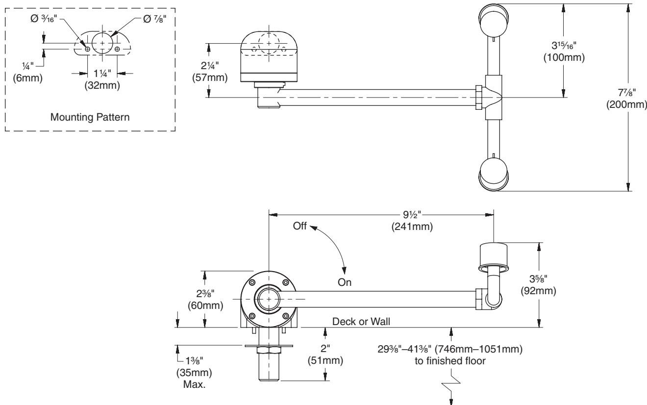
**Dimensions — S19274HD, S19274HDR, S19274HW** (deck-mounted unit shown)
