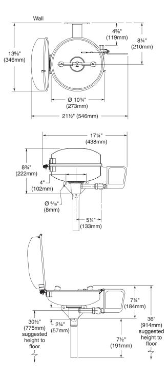
All dimensions assume standard thread engagement. Variations in manufacturing allow for +/- 1/8" (3mm) per threaded joint. To find the tolerance of a dimension, add the number of thread joints in between a dimension and multiply it by 1/8" (3mm).
