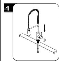
Optional Flange Installation: Before installation, ensure that the flange (1) is placed on the bottom of the new faucet assembly. Insert the faucet body through the hole in the sink.
