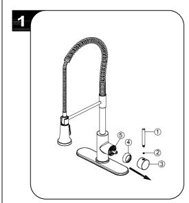
Shut off water supply. With valves in "closed" position, remove handle (1) from handel seat (3). Loosen the set screw (2) and unscrew the cap (4) from the cartridge nut (5).
