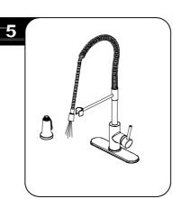
Important: after installation is completed, turn on hot and cold water supplies. Check for leaks. Remove the spray head by unscrewing it from the hose counterclockwise. Be sure to hold the end of the hose down into the sink and turn the faucet on to the warm position where it mixes hot and cold water. Flush water lines for one minute. Check for leaks. Re-tighten any connections if necessary, but do not overtighten. Reinstall spray head by hand tightening it back onto the spray hose.
