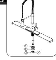
Secure the faucet assembly with the washers (1&2) and nut (3). Hand tighten the nut (3) onto the faucet assembly. Lock the nut (3) into position by tightening the screws (4) with a phillips screwdriver.
