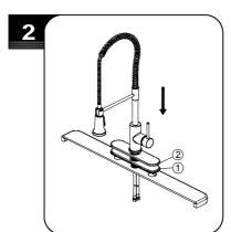
Optional Deck Plate Installation: Before installation, align the hole in the gasket (1) and deck plate (2) with the mounting hole in the sink. Place the faucet assembly through the deck plate (2) and mounting hole in the sink until the faucet assembly sets on top of deck plate (2). NOTE: If the sink is uneven, use silicone
