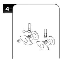
Make connections to water lines. Thread the nut (1) on the supply line onto the outlet of the water supply valve (2) and tighten with a wrench. Do not overtighten.
