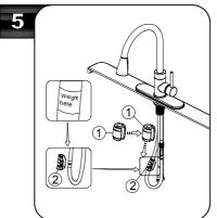
Install the weight clip (2) at the point of the hose marking "Weight here".
