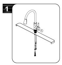
Optional Flange Installation: Before installation, ensure that the flange (1) is placed on the bottom of the new faucet assembly. Insert the faucet body through the hole in the sink.
