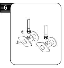
Make connections to water lines. Thread the nut (1) on the supply line onto the outlet of the water supply valve (2) and tighten with a wrench. Do not overtighten.
