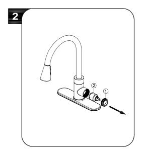
Loosen cartridge nut (1) by turning it counter-clockwise and lift out the cartridge (2). Insert new cartridge. Reinstall the handle.
