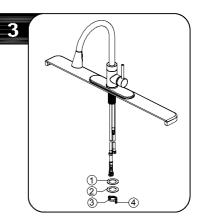
Secure the faucet assembly with the washers (1&2) and nut (3). Hand tighten the nut (3) onto the faucet assembly. Lock the nut (3) into position by tightening the screws (4) with a phillips screwdriver.
