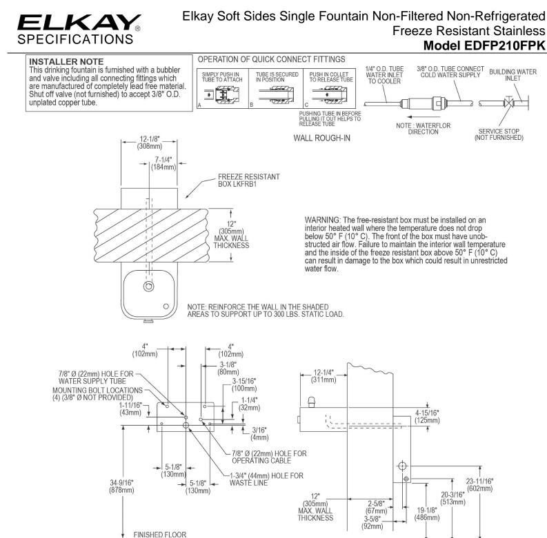
NOTE: ALL DIMENSIONS ARE TAKEN FROM THE FINISHED FLOOR ON THE SIDE OF THE WALL THAT THE FOUNTAIN IS ON.
