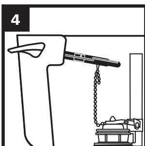
**Connect flapper to arm hole. Chain needs slight slack (small J shape) when flapper is in closed position. Test for proper flush and adjust slack if needed. Tighten locknut by hand. DO NOT overtighten as it may crack tank.**
