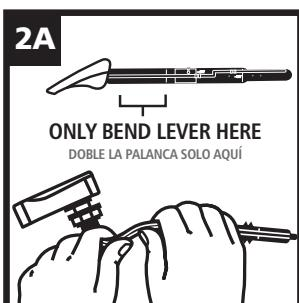
**For side or angle-mount:** slowly bend new lever arm to match shape of old lever arm. (See picture where to bend lever). DO NOT bend arm quickly or back and forth repeatedly.
