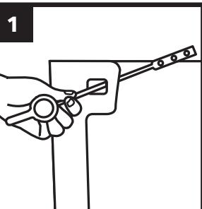
**Remove tank lid. Disconnect flapper from lever. Unthread nut from old lever. Remove lever from tank.**
