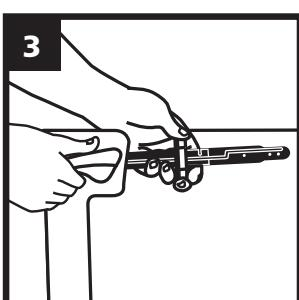
**Slide arm through tank hole until handle fits snugly. Slip lock nut over lever arm (flat side facing handle). Place nut on threads, turn counter-clockwise (reverse thread) to hold in place. DO NOT tighten fully.**
