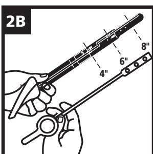
**For front mount:** measure length of existing lever arm. Match new arm length to old arm (may need to trim at cut line. Hacksaw recommended).
