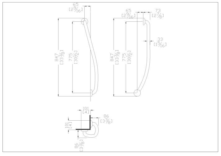
Two wall transition grab bar. No maintenance 3mm thick antimicrobial vinyl coating. Concealed stainless steel 11-hole flange plate.
