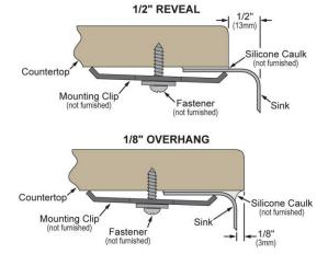
Designed to affix to the underside of any solid surface countertop.
