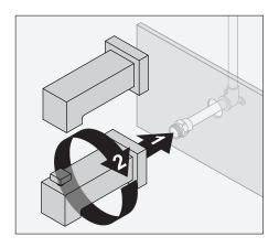
3) Thread tub spout (361TS or 361DTS) onto fitting.
