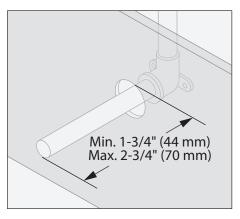
1) Rigid copper tubing must protrude 1-3/4" (44 mm) - 2-3/4" (70 mm) from finished wall.
