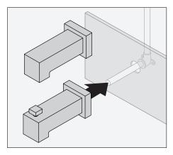
2) Attach tub spout (361TS or 361DTS) to rigid copper tubing.
