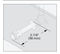
1) Male 1/2-14 NPT fitting must protrude 3-7/8" (98 mm) from finished wall
