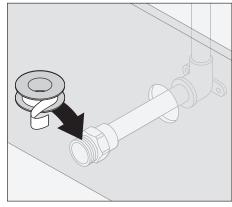
2) Apply plumber tape to threads on fitting.
