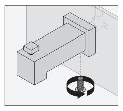
3) Install set screw to secure tub spout to rigid copper tubing.
