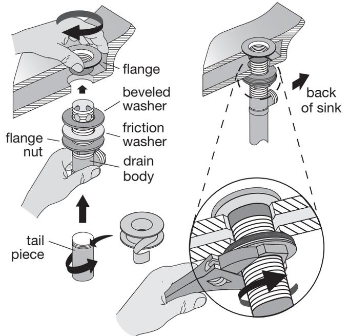
\* Note: Attach tail piece to drain body using teflon tape, tape or plumber's putty.
