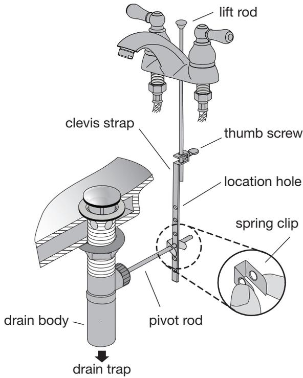
**Step 8 Attach drain body to drain trap**
