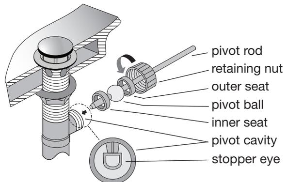
**Step 7 Connect lift rod and adjust linkage**
