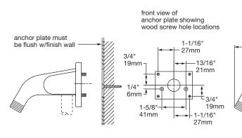
Anchor plate used for ceramic tile application—plate screws to wall and tile is applied up to sides of plate. Mounting bracket is mounted on finished wall with machine screws into anchor plate
