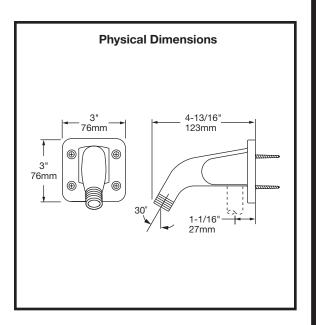
Installation with Anchor Plate - Suffix "A"
